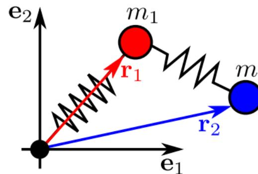
model of mechanical system: two concentrated masses
